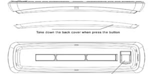
The receiver on the slot of the back cover
